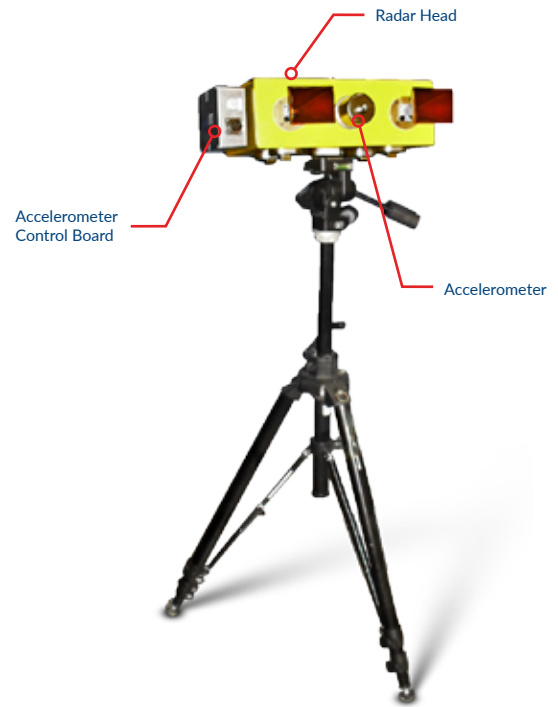
IBIS-FS Plus Incorporates an Accelerometer
