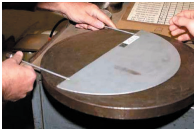
Figure 4 - Calibration of a flat jack.
