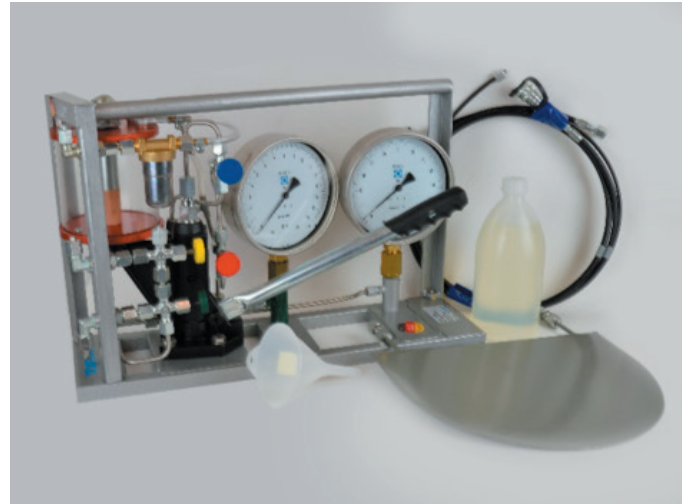
Figure 1 - Flat jack testing equipment.
