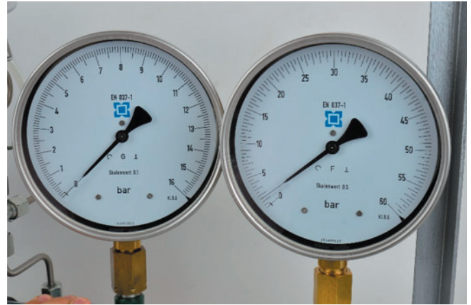
Figure 8 - M2H16 pump precision gauges.
