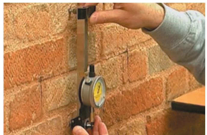
Figure 7 - Application of the DEMEC deformometer.
