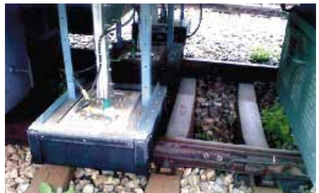
SRS configured with antennas beneath the train
