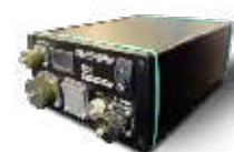
SRS Radar control unit
