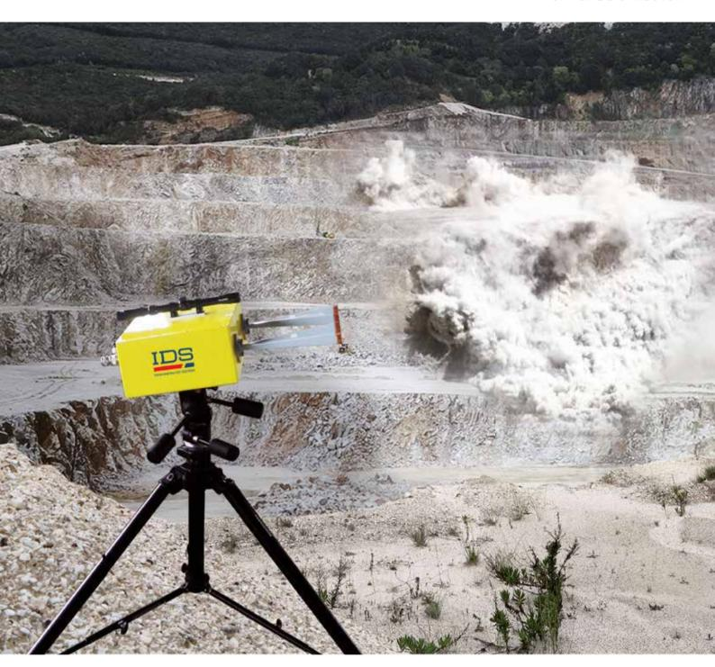
Interferometric radar for broad area monitoring of blast-induced vibrations
