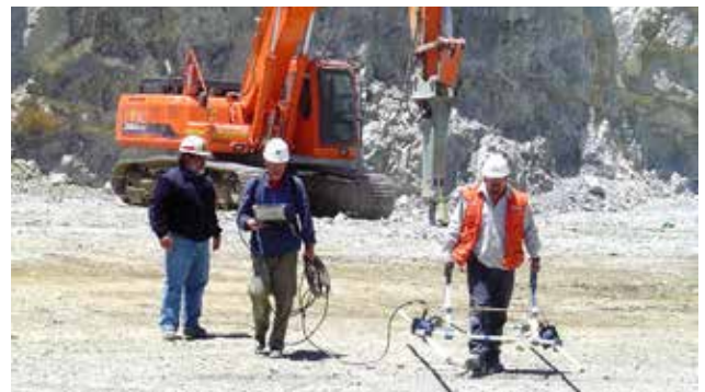
Survey with a low frequency antenna at a mine
