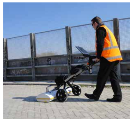
RIS Hi-BrigHT: pavement surveying
